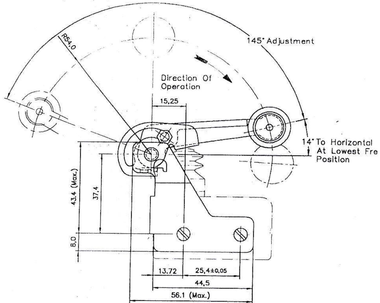
Auxiliary actuator for optional use with Standard Size Enclosed terminal
